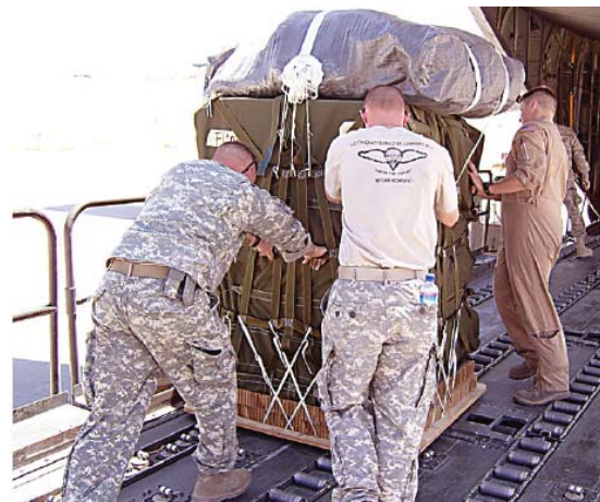
Containerized delivery system (CDS) bundles are loaded onto a C-130 or C-17 aircraft, where riggers will jointly inspect the bundles with Air Force personnel before handing over the airdrop mission.
